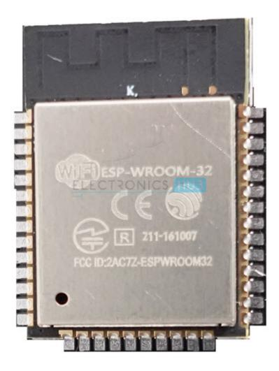
The good thing about ESP-WROOM-32 Module is the PCB has edge castellations. So, what third-part manufacturers do is take the ESP-WROOM-32 Module and design a break-out board for this module.
